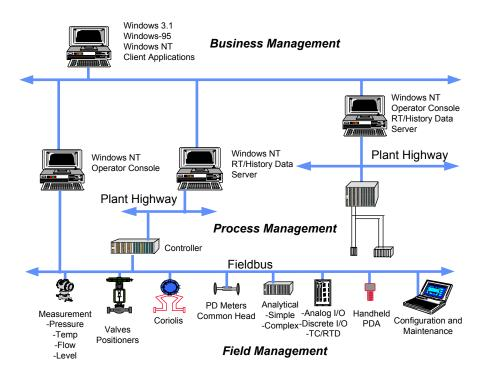
Figure 1-1 Process Control Information Architecture
