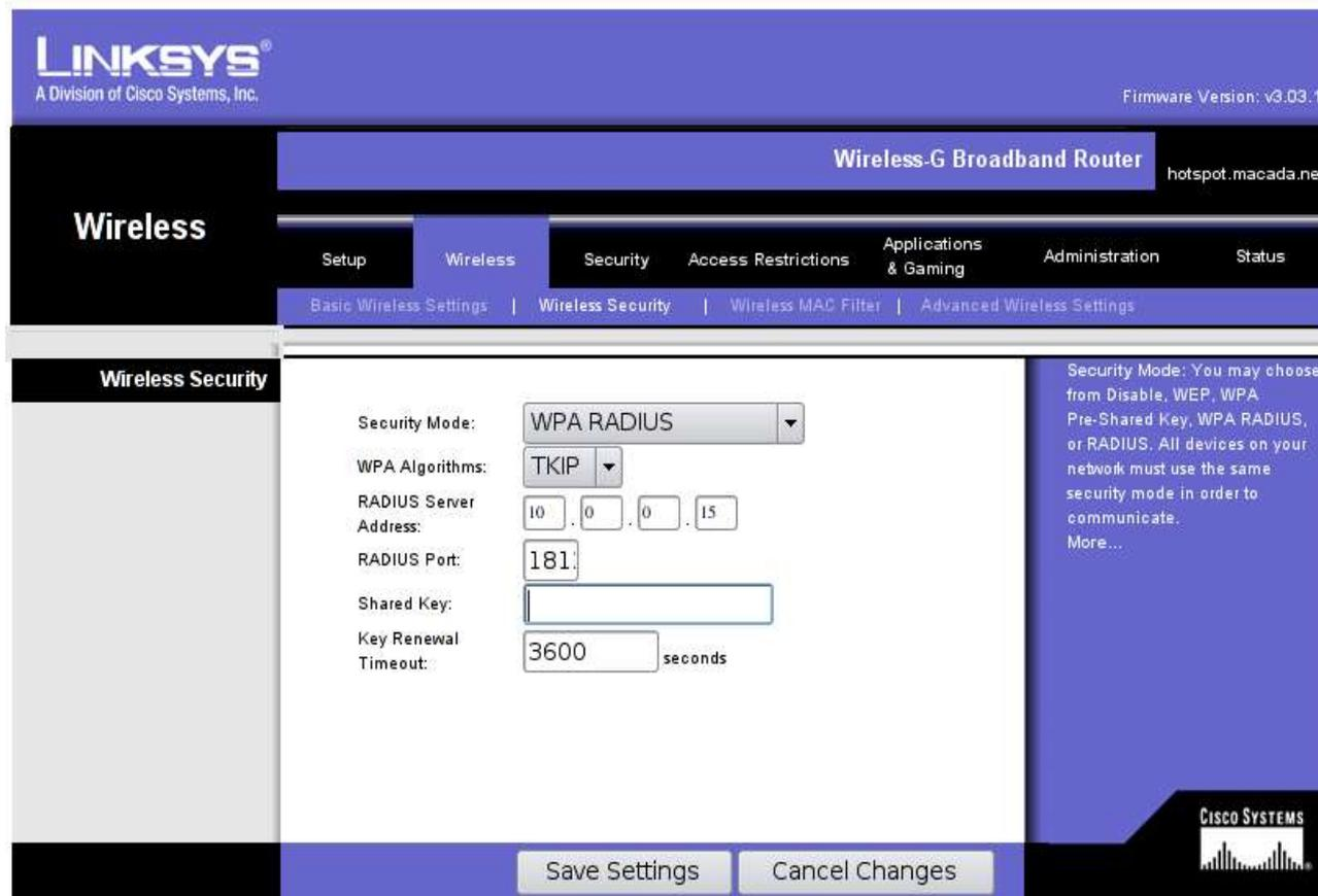
The screenshot shows the Linksys configuration interface for a Wireless-G Broadband Router. The page is titled "Wireless Security" and is part of the "Wireless" section. The "Security Mode" is set to "WPA RADIUS". The "WPA Algorithms" are set to "TKIP". The "RADIUS Server Address" is "10.0.0.15" and the "RADIUS Port" is "181". The "Shared Key" field is empty, and the "Key Renewal Timeout" is set to "3600 seconds".
